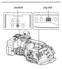
Tilt the joystick or turn the jog dial to set the cursor to "Date/Time" then press the joystick or dial.
